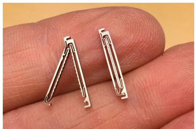
Nitinol clip. Thinnest segments 0.1 mm. Tolerance \pm 10 \mu\text{m} .
